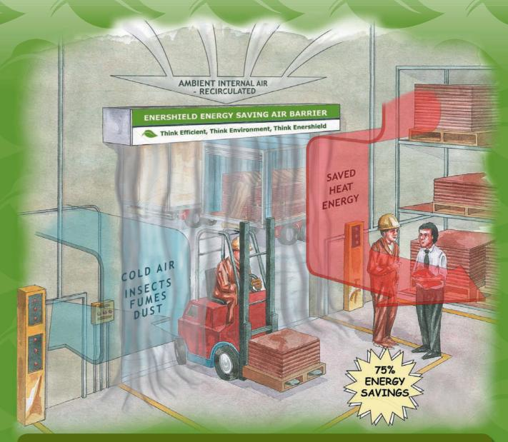
Creates up to a 90% seal on open doors by recirculating facility air
