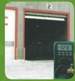
Plus 14°c inside and minus 23°c outside after one hour with the door open.
