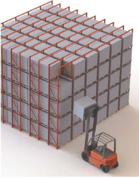
RediRack drive-in racking provides storage for pallets whilst using a minimum of floor space. It offers the same goods protection and preservation as other rack applications but with reduced selectivity. Any standard reach or counterbalance truck is suitable for use with the system.
