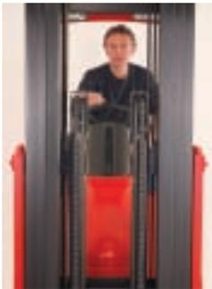
Operators have superb forward visibility thanks to the triplex free lift mast, with its twin side mounted lift cylinders. Mast tilt design means easy fork entry into pallets – even over trailer retaining rails.
