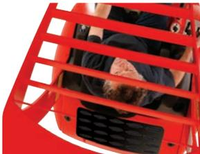
The unique 'Hi Vis' twin post safety guard combines maximum visibility and overhead protection for the operator.
